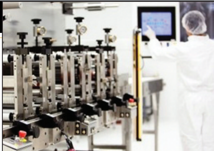
Fabrico has three Class 10,000 clean room facilities for medical packaging converting and assembly.
