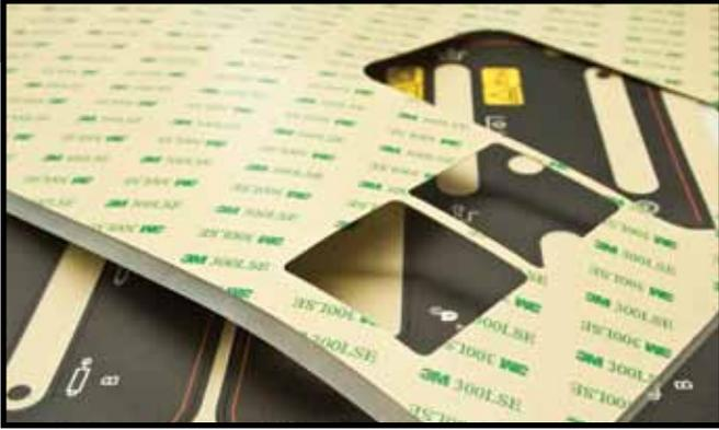
Liquid adhesives, adhesive tapes, and thin film/foam bonding systems create strong bonds with LSE plastics that are more resistant to impact, shock, and fatigue than conventional mechanical and ultrasonic fastening.
