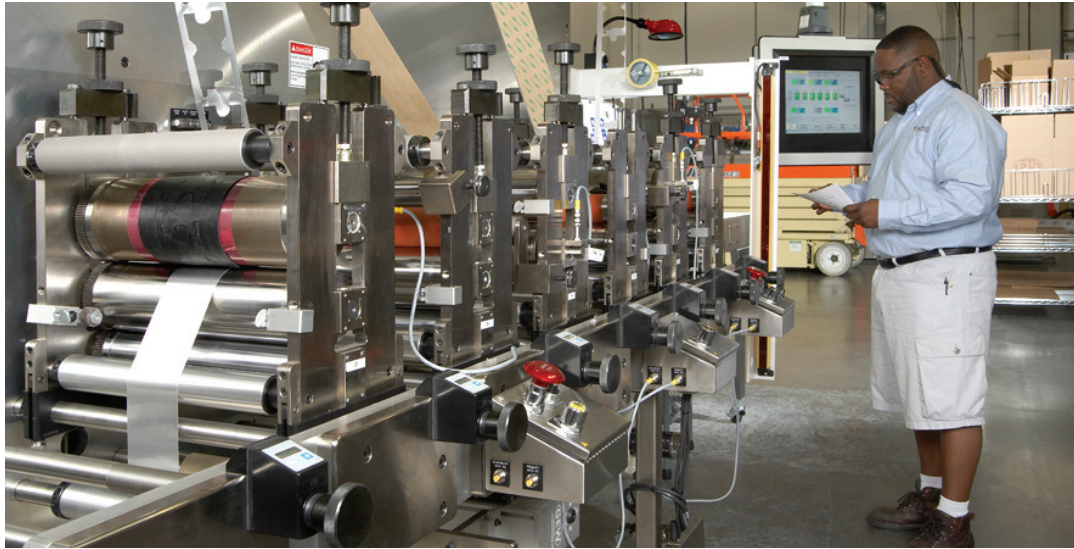
Fabrico's Delta Rotary Press at the company's Kennesaw, GA facility, used for die cutting, laminating, and single-color printing.
