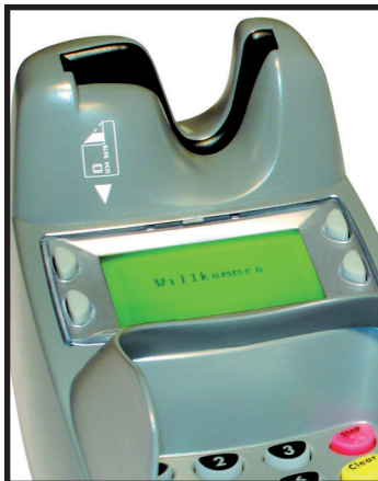
To meet industry, consumer, and regulatory demand, Ingenico designed a PIN pad shroud for payment terminals.
