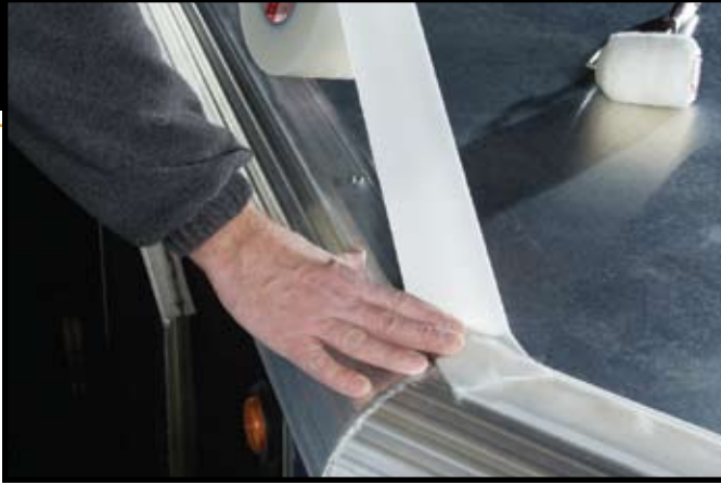
Pressure-sensitive foam tapes and adhesive transfer tapes can accommodate expansion/contraction cycles.
