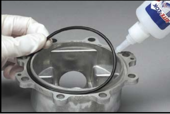
Acrylics provide fast curing, high-strength bonds for a range of substrates without surface preparation.
