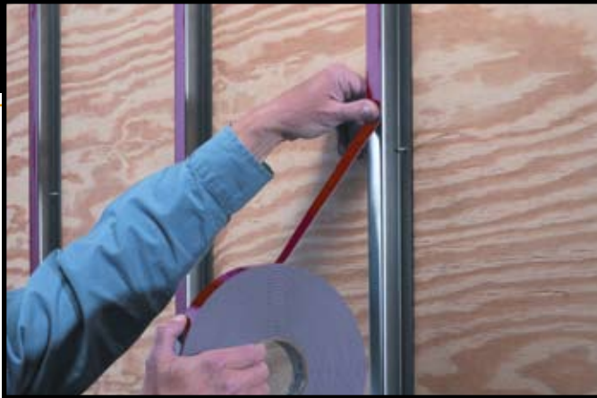
Tapes are used worldwide instead of rivets, screws, or other mechanical fastening systems.
