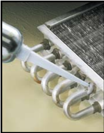
Liquid adhesives are replacing mechanical fasteners where high strength and structural integrity are requirements.
