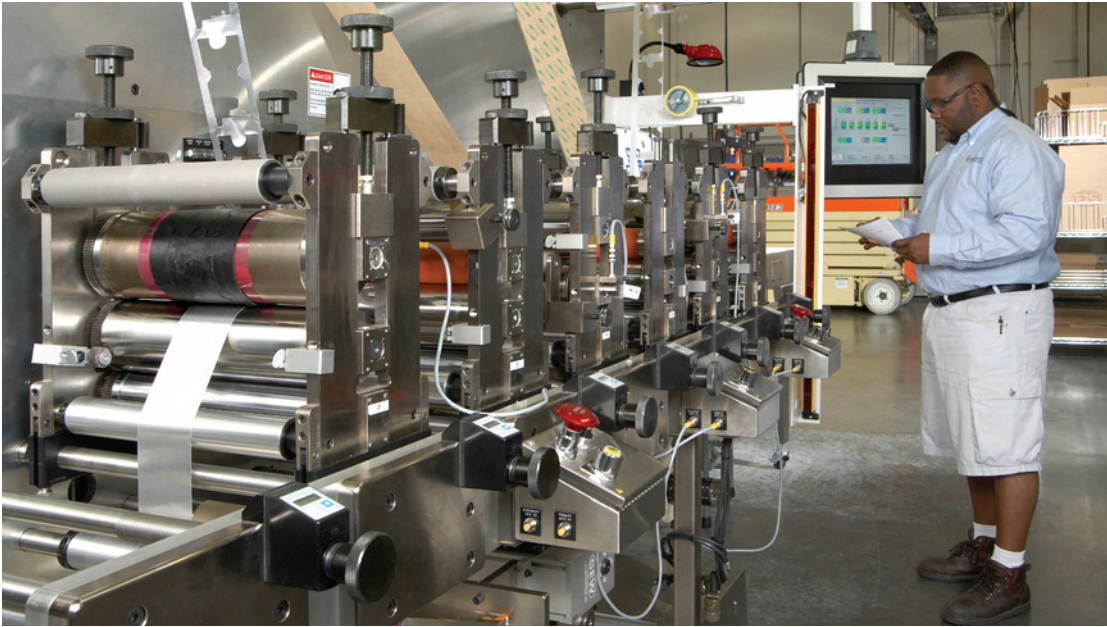
Fabrico's Delta Rotary Press at the company's Kennesaw, GA facility, used for die cutting, laminating, and single-color printing.
