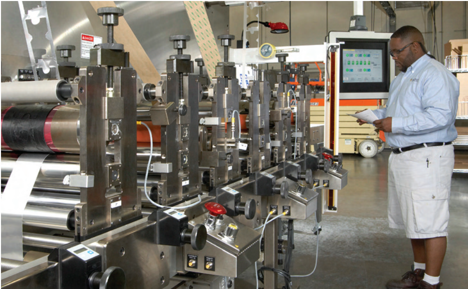
Fabrico's Delta Rotary Press at the company's Kennesaw, GA facility, is used for die cutting, laminating, and single-color printing.
